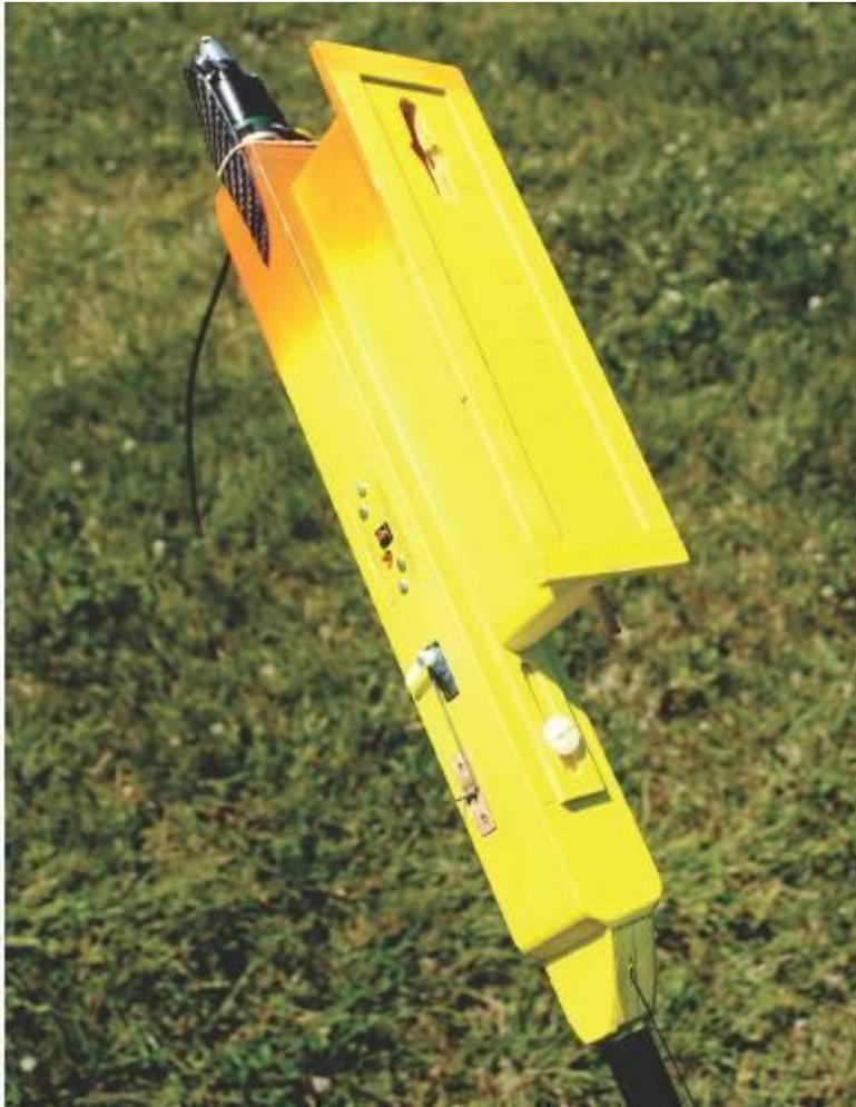
Above: Loosening two 1/4-20 screws on Dale's model allows the pylon to be moved forward or back. Removing the wing allows access to the front screw; the rear screw goes into a slotted tab attached to the rear of the pylon.
