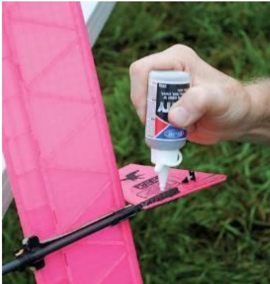
A product used by model railroaders called Liquid Gravity also works for fine-tuning a FF model's CG. Simply sprinkle it onto slow-curing CA glue.
