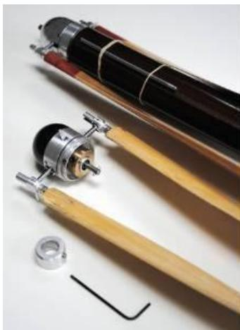
Removable weights on this F1B Rubber model allow the CG to be moved forward for windy conditions. The brass one weighs approximately 8 grams and the aluminum one is roughly 4 grams.
